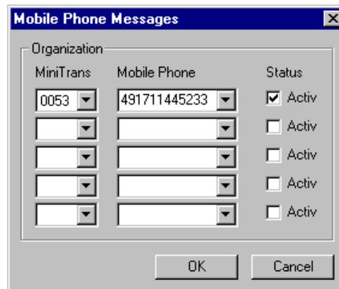
All MiniTrans sensors registered in the WinTrans database are listed in the "**MiniTrans**" column. Select the serial number of the MiniTrans sensor the measured values of which shall be transmitted to a mobile phone. Enter the mobile phone number in the usual format in the "**Mobile Phone**" column. Mark the "**Status**" check box .
