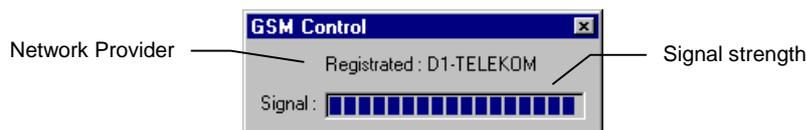
The entire GSM signal test lasts approximately 3 minutes and will then be terminated by MiniTrans automatically.
