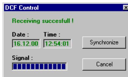
Click the "Synchronize" button to synchronize the internal MiniTrans clock with the current DCF time.
