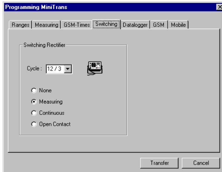
Cycles 4/2, 12/3, 27/3 and 57/3 are available. These 4 different switching cycles are not wired in the Mini-Trans but defined by the WinTrans software. It is thus guaranteed that other switching cycles can be added by the manufacturer in the WinTrans software in case of new kinds of intensive measurements or maintenance processes without changing the MiniTrans devices at site.
